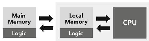
**Figure 1** Logic-in-memory computing paradigm: application-specific logic for localized computation is hidden behind a memory abstraction.
